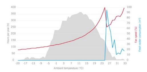
▲ Water supply is required only during a few hours in the course of a year. It immediately reduces the fan speed. This is because adiabatic pre-cooling lowers the temperature level of the air as the water in the pads evaporates, thereby removing energy form the ambient air.
